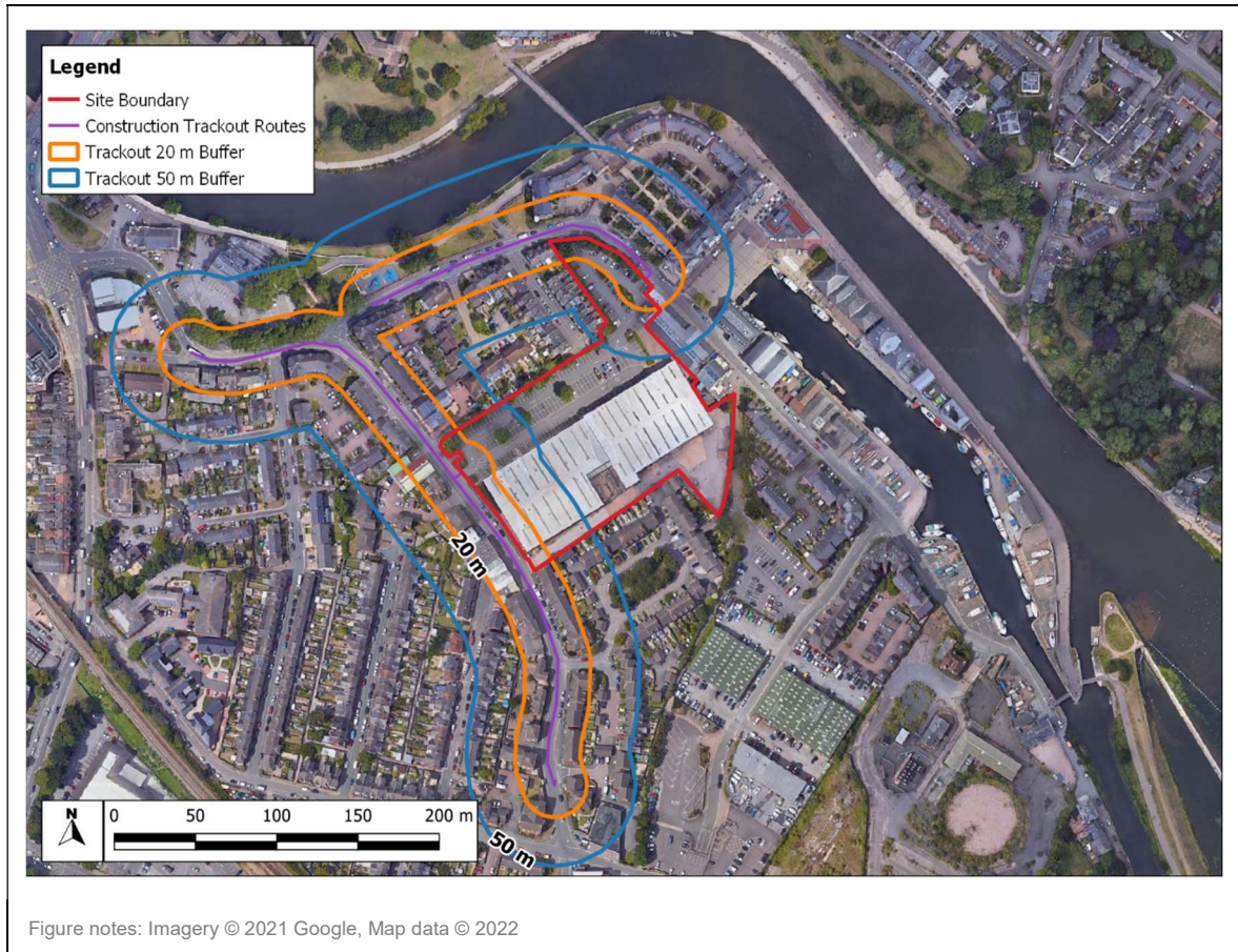
Figure 7: Distance Buffers from Road Lanes where Dirt may be Tracked out from the Site
