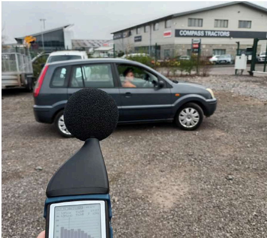
Figure 8: Photograph of sound measurement being made as the car moving across the gravel surface
