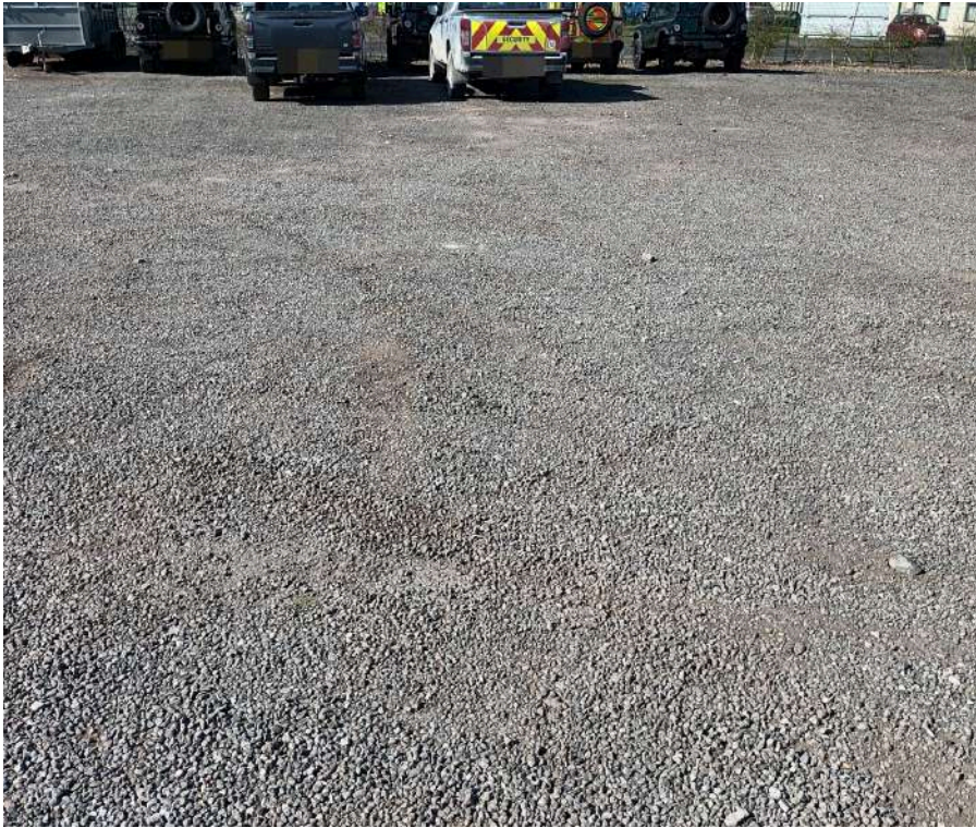
Figure 9: Photograph of the unbound gravel surface on which the measurements were taken
