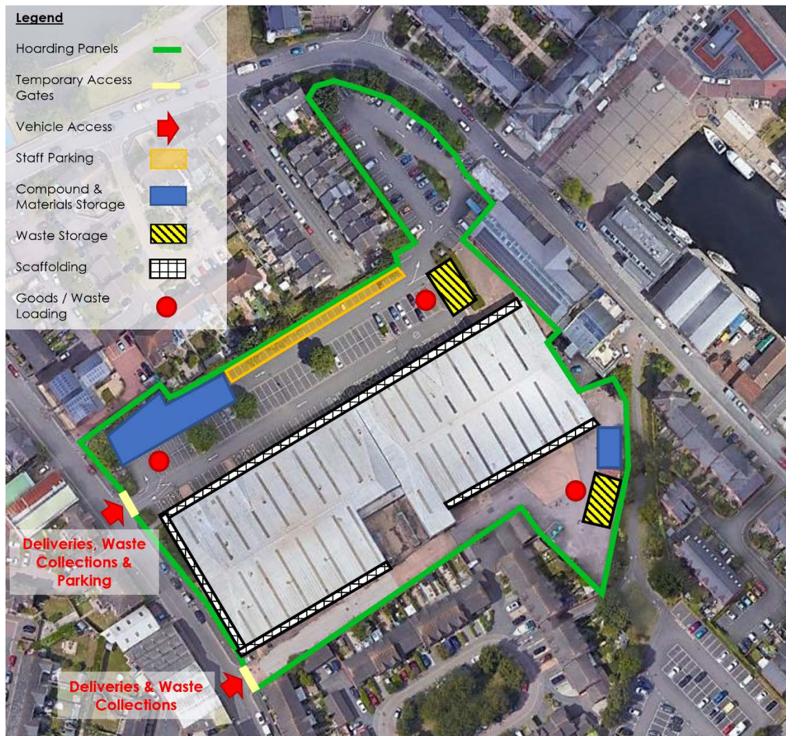
Figure 4 Indicative Demolition Set-Up
