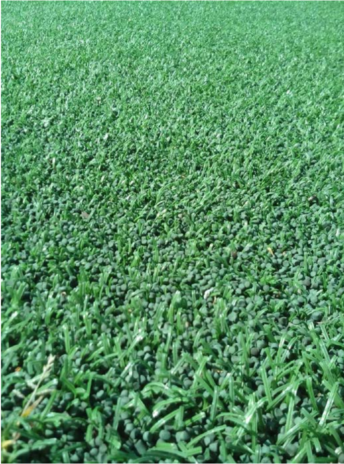
Figure 4. 3G artificial turf with TPE pellets acting as performance infill (Gothenburg, Sweden)
