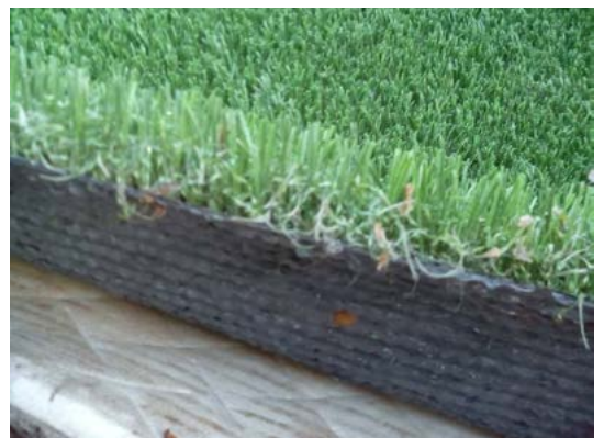
Figure 8. A non-infill design, with underlying shock pad
